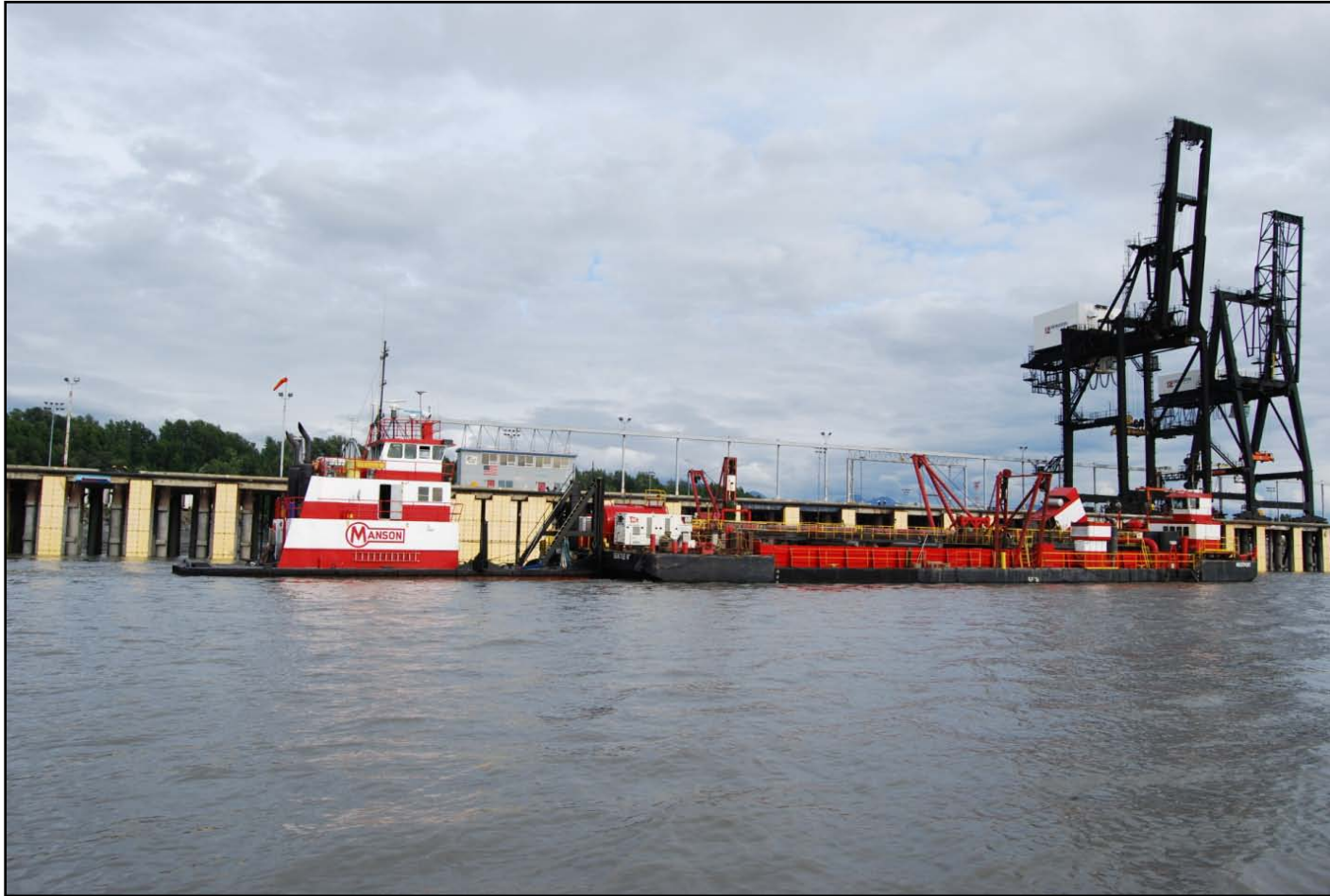
Figure 13. Suction dredge operating at the Port of Anchorage.
